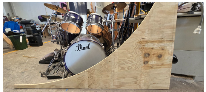
CNC-cut transition profile at Blink Design.
